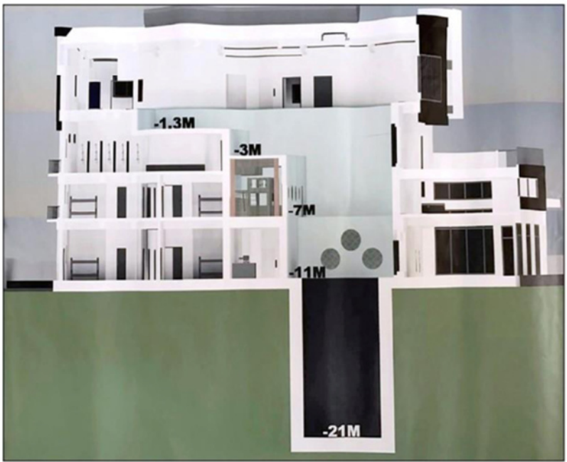
Figure 1 The building section of Divecube Hotel. The pool has five various depth levels, with the deepest one being measured at 21 meters
